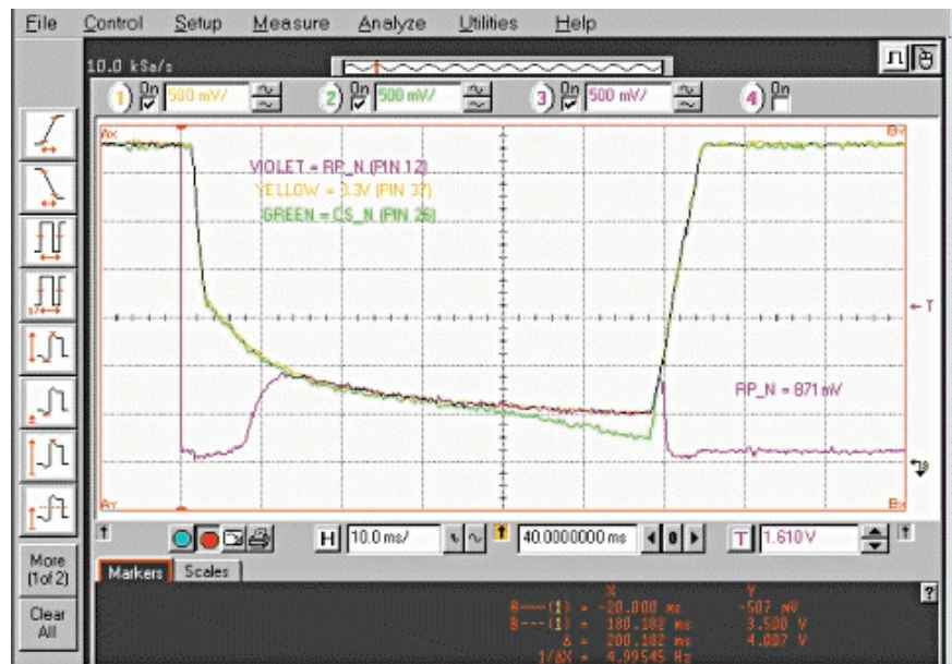
Figure 3. With a standard high-speed scope, the analog behavior of the signals becomes apparent, but the chip select activity expected after RP_N went high was nowhere to be seen.
